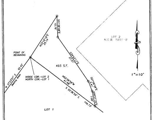
The plat as shown herean was prepared from an on—the—ground survey performed under my supervision during the month of April, 2007.
